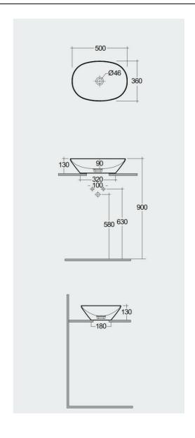
Dimensions: All dimensions in mm. Tolerance of vitreous china & fireclay items:  $\pm$  5% for below 200mm and  $\pm$  3% for above 200mm; for all other items tolerance  $\pm$  1%. Note: Due to a continuing development program to improve design and performance, the manufacturer reserves all rights to vary specifications without prior information. Please note accessories are for photographic use only.
